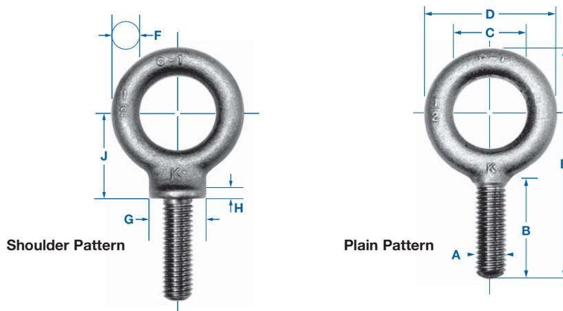
**Caution:** Rated capacity is for 0° vertical pulls. See Eyebolt Rated Capacity/Guidelines (page 7) for complete lifting information. Reference ASME B18.15 for additional dimensions. Swivel Hoist Rings (page 63) are recommended for angular lifts.
