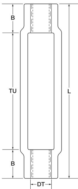
Turnbuckle body specimens conform to the physical requirements of ASTM F1145.
