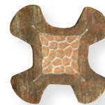
Indenter Crimp Cross-Section Across Axis
