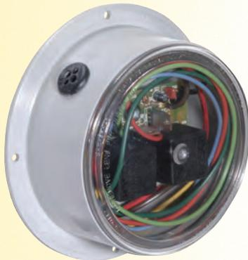
A high capacity flasher that can flash a maximum lamp load and hold a constant flash rate regardless of voltage variations or number of lamps, plus, the actuator signal switch receives less than one amp. Other features include instant start and immunity to motor transient noise. 12" pigtail included. Wiring diagram included. Surface mount.
