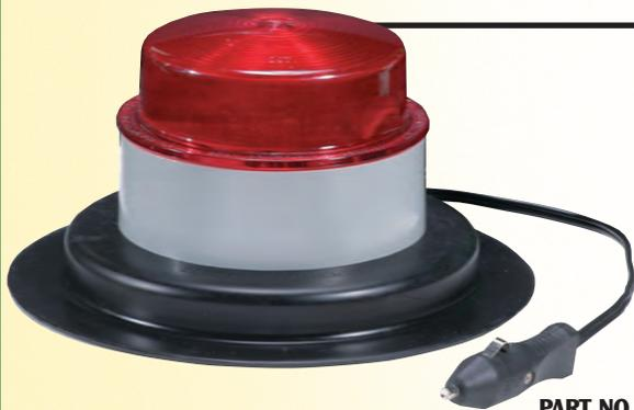
Strobe featuring high impact valox housing and polycarbonate lens. The Xenon flash tube with a life of 10 million flashes produces an (8) joule output per flash. Has a flash rate of 70 flashes per minute and an effective candle power of 102 with clear lens. Consumes 1 amp at 12 volts. Includes suction gasket, magnet, 8' of wire and cigarette lighter adapter.
