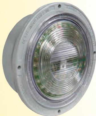
Back up lamps are available in incandescent multi and single diode, and both are Multi-voltage. LED lamps are designed to operate for either 12 or 24 volt systems. Incandescent lamps use a 920139 lens with a 920460 socket and 1156 bulb. Multi-diode lamps use a 710037 LED clear lens assembly and the single diode lamp uses a 920139 lens with a 920691 single diode LED assembly.
