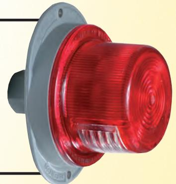
A self grounding valox body lamp that features a 920113 lens. Uses a 920127 socket and 67 bulb. Provided with a 1/4" N.P.T. rear entry. Surface mount.
