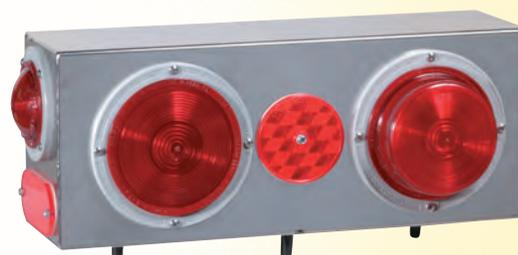
**435006** Curb side module consists of a marker lamp, turn/tail, stop/tail. Module is provided with 10-1/2' of 4 conductor cable (red, white, green, brown) and (3) 1-14 x 15 mounting studs are welded to the bottom of the module for installation. Module has two reflectors installed. Frame only part number is 920591.
