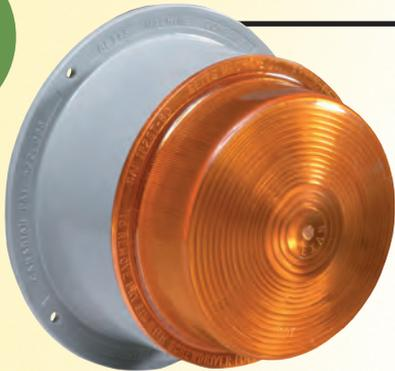
Strobe featuring high impact valox housing and polycarbonate lens. The Xenon flash tube with a life of 10 million flashes produces an (8) joule output per flash. Has a flash rate of 70 flashes per minute and an effective candle power of 102 with clear lens. Consumes 1 amp at 12 volts. Mounting gasket, screws and 8" pigtails included.
