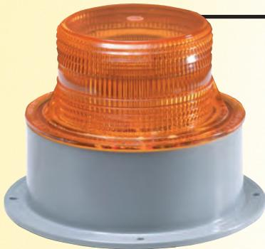
Halogen beacons may be used in place of strobes for many applications. Halogen beacons feature a tough valox housing and polycarbonate high hat lens. Simplified circuitry along with good shock resistance insures less maintenance. The Halogen bulb is field replaceable. Mounting gasket, screws and 8" pigtails included.
