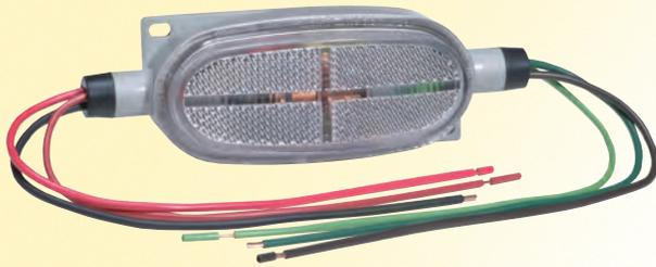
Betts circuit saver protects flasher circuits when extra lamp loads are used. It also extends switch life. Lamp loads of up to (24) 32 c.p. bulbs or 60 amps for both 4 and 7 wire 12 volt systems can be handled. Contains high quality Palladium relay contacts and has positive or negative ground. The Valox housing uses a clear 920143 shallow polycarbonate lens and is prewired with 12" pigtailed. Mounting gasket, screws and wiring diagram are included. Surface mount.
