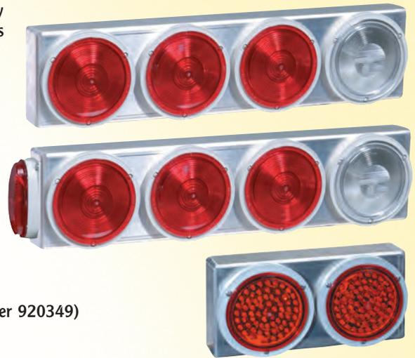
Lamp bodies are 45 series valox and are available in incandescent bulb, 12 volt multi-diode, or Multi-voltage single diode stop, turn or tail lamps. Side markers are 12 volt incandescent bulb or 12 volt LED with a reflective lens. Both LED versions come as a double contact but can be converted to a turn only function by dead heading the tail/clearance marker wire in the body.
