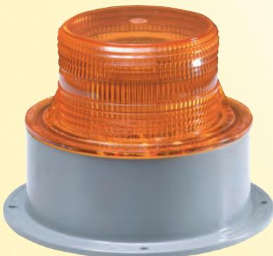
Strobe featuring high impact valox housing and polycarbonate lens. The Xenon flash tube with a life of 10 million flashes produces an (8) joule output per flash. Has a flash rate of 70 flashes per minute and an effective candle power of 102 with clear lens. Consumes 1 amp at 12 volts. Mounting gasket and screws included.
