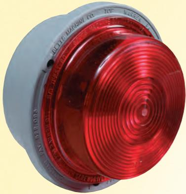
Strobe featuring high impact valox housing and polycarbonate lens. The Xenon flash tube with a life of 10 million flashes produces an (8) joule output per flash. Has a flash rate of 70 flashes per minute and an effective candle power of 102 with clear lens. Consumes 1 amp at 12 volts. Mounting gasket, screws and 8" pigtails included.
