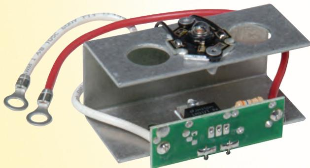
A high output Multi-voltage single LED assembly. Assemblies meet F.M.V.S.S. 108 compliance for stop/turn/tail or marker functions while operating within a voltage variance range from as little as 8 volts to as high as 44 volts without degrading the LED or circuitry. Assemblies all come as a double contact but can be wired internally to meet any functions needed.
