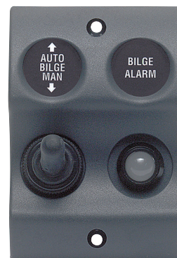
900-BA Bilge alarm and bilge pump control panel includes: 1 on/ off/on switch for auto manual control; 1 warning light and alarm for high water level alarm. (Float switch ordered separately - Part # SB1-FS)
